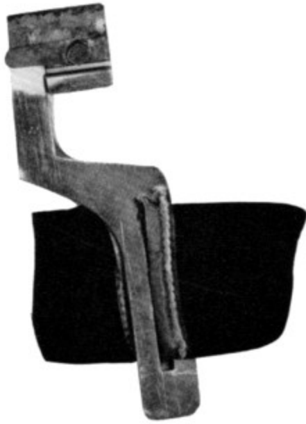
Figure 61.—SPOUL'S patent braid guide, 1871. (Smithsonian photo P-63102.)
