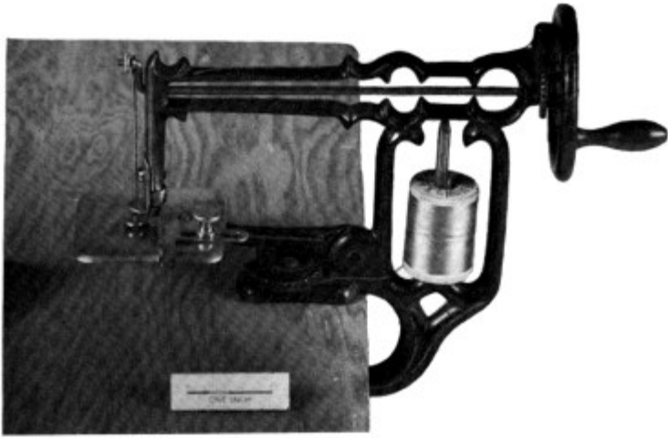
Figure 93.—HANCOCK SEWING MACHINE, 1867. One of the many inventors who turned his talents to inventing and producing a mechanically simple and cheaper machine was Henry J. Hancock. His 1867 machine is only about six inches wide; it uses a tambour-type needle, pulling a loop of thread from below the stitching surface. (Smithsonian photo P63197.)
