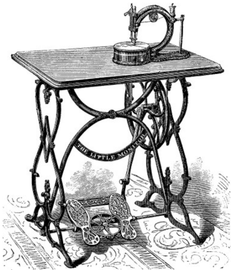
Figure 80.—DU LANEY SEWING MACHINE of about 1872. Most of the small, simple, chainstitch sewing machines of this period were constructed so that they could either be turned by hand or set into a treadle-powered table. Du Laney's Little Monitor, manufactured for only a few years, was based on the patents of G.L. Du Laney, July 3, 1866, and May 2, 1871. It was a two-thread, chainstitch machine powered only by a foot treadle. By simple
