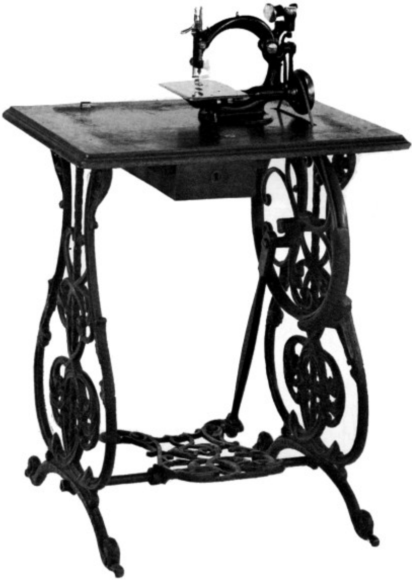
Figure 131.—WILLCOX AND GIBBS SEWING MACHINE, serial number 296572, of about 1878. From 1857 to the turn of the century, the style of the Willcox and Gibbs sewing machine changed very little (fig. 39). It was the most popular and the most reliable
