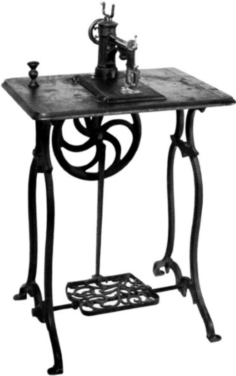
Figure 127.—WEST & WILLSON SEWING MACHINE of about 1859. The West & Willson machine, manufactured under the patent of H. B. West and H. F. Willson, enjoyed a very brief span of
