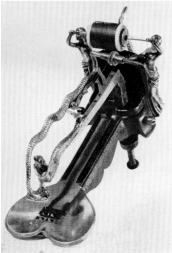
Figure 46.—IN ADDITION TO MECHANICAL PATENTS, a number of design patents were also issued for sewing machines. These fall into a separate series in the Patent Office's numerical records. This unusual example featured two semidraped female figures holding the spool of thread, a mermaid holding the needle, a serpent which served as the presser foot, and a heart-shaped baster plate. The design was
