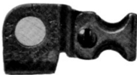
Figure 56.—HARRIS' patent thread cutter, 1872. (Smithsonian photo P-6397.)
