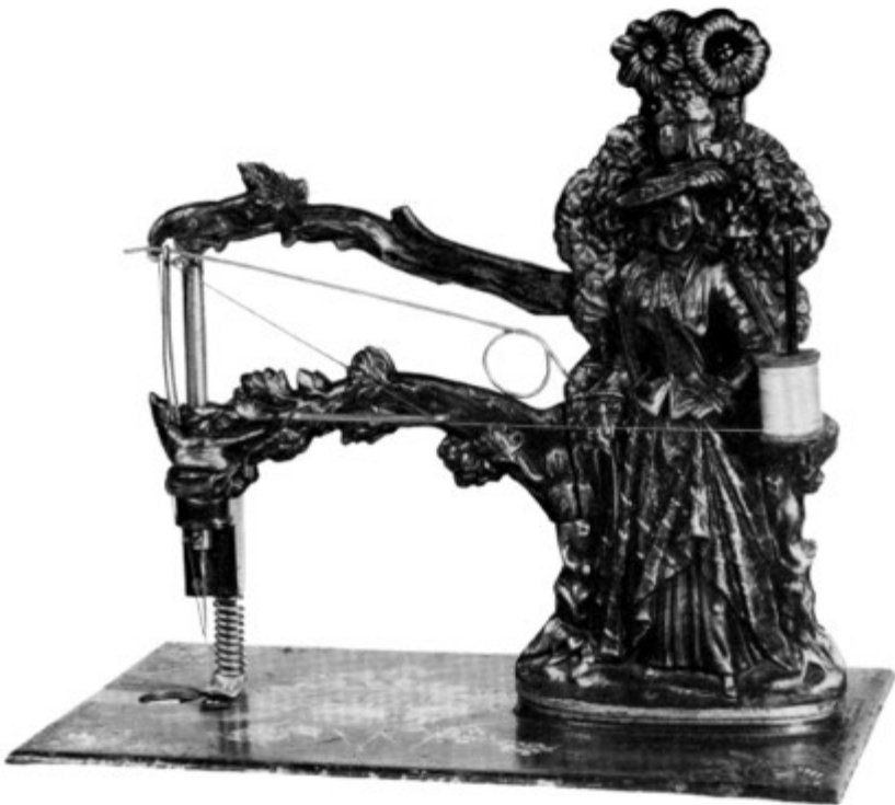
Figure 104.—“LADY” SEWING MACHINE of about 1859. The contemporary name of this machine is unknown. The unusual design of the head, or main support, is based in part on the design patent,
