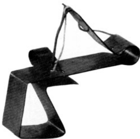
Figure 48.—HEYER’S POCKET SEWING MACHINE patent model, November 17, 1863. This patent model is one piece, and measures about two inches in height and two inches in length. It will stitch—but
