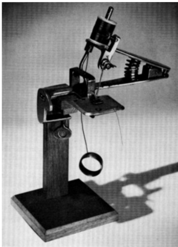
Figure 75.—BECKWITH SEWING MACHINE, 1871. Among the inventors whose patent claims were “to produce a cheap and effective sewing machine” was William G. Beckwith. His machine was first manufactured by Barlow & Son, and it realized considerable success in the few years of its production. The earliest model was operated like a pair of scissors or with a cord and ring as illustrated. Beckwith later added a hand crank. The machine was purchased in Crewe, Cheshire, England; it is stamped “Pat. April 18, 71 by Wm. G.
