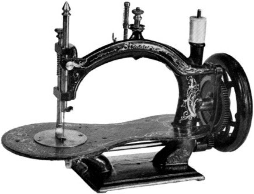
Figure 123.—STANDARD SEWING MACHINE of about 1870. This chainstitch machine is believed to have been made by the company that later became the Standard Shuttle Sewing Machine Company, when they began manufacturing lockstitch machines about 1874. This machine is marked with the name, “Standard,” and with the dates “Patented July 14, 1870, Patented Jan. 22, 1856, Dec. 9, 1856, Dec. 12, 1865.” The dates refer to the reissue and extended reissue of the Bachelder and the A. B. Wilson patents. The number of chainstitch
