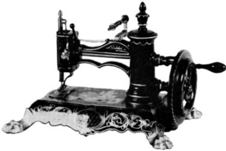
Figure 89.—WILSON SEWING MACHINE, late 1860s to early 1870s. In addition to the Buckeye (see fig. 77), W. G. Wilson manufactured several other styles of sewing machines. This one, a combination of the varying styles of the earlier pillar machine has even duplicated the general style of the spool holder patented by Folsom. The pillar is not striated, but the machine does repeat the claw feet of the Atwater and Monitor machines. Wilson machines are usually marked “Wilson Sewing Mach. Manuf’g Co. Cleveland, Ohio, Ketchum’s Patent April 28, 1863.” The latter name and/or patent date are found on many of the machines of this general construction. The patent is that issued to Stephen C. Ketchum for his method of converting rotary motion into reciprocal motion.
