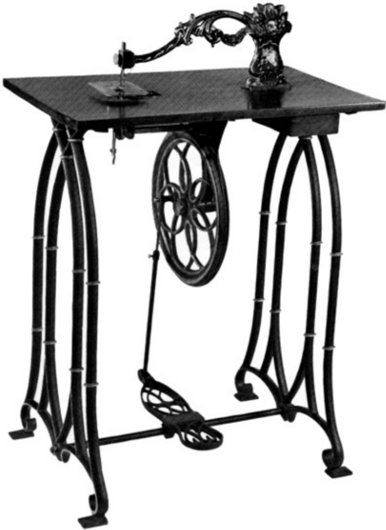
Figure 105.—LANDFEAR'S PATENT SEWING MACHINE of about 1857. Another of the many machines that, except for isolated examples, have almost completely disappeared from the records is Landfear's machine. Fortunately, this
