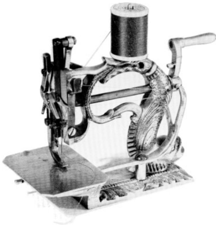
Figure 40.—A DOLPHIN sewing machine based on Clark's patent of 1858. This design was first used by T. J. W. Robertson in 1855, but in his patent issued on May 22 of that year no claim was made for the machine design, only for the chainstitch mechanism. The same style was used by D.
