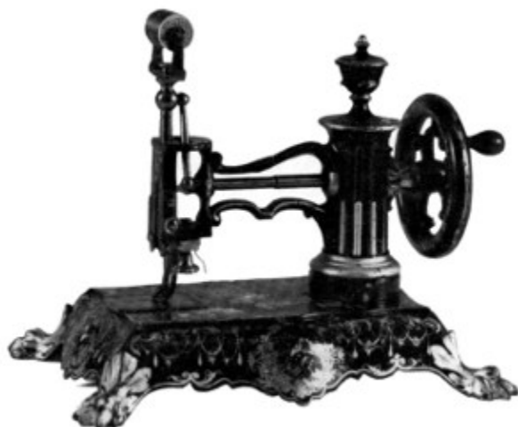
Figure 87.—ATWATER SEWING MACHINE, 1858. Atwater machines, based on the patent of B. Atwater, issued May 5, 1857, were manufactured from 1857 to about 1860. The machine illustrated, which is designed to be operated by a hand-turned wheel, has an upper forked dog feed, and its horizontally supported spool is directly over the stitching area. Like the others, it has a striated pillar and claw feet. The manufacturer is unknown. (Smithsonian photo P63200.)
