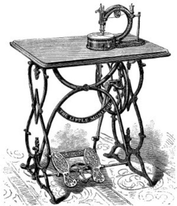
Figure 80.—DU LANEY SEWING MACHINE of about 1872. Most of the small, simple, chainstitch sewing machines of this period were constructed so that they could either be turned by hand or set into a treadle-powered table.
