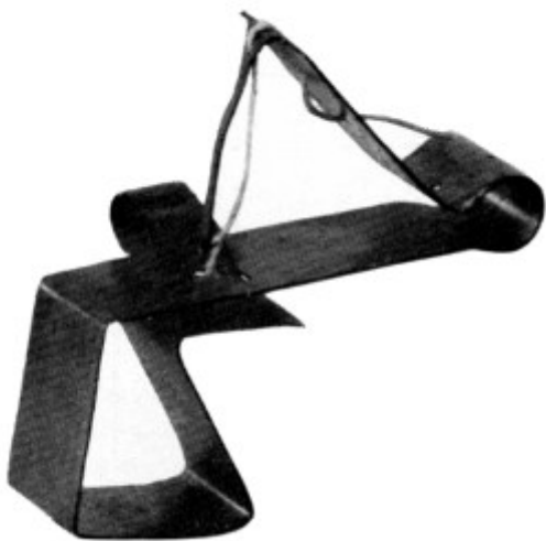
Figure 48.—HEYER'S POCKET SEWING MACHINE patent model, November 17, 1863. This patent model is one piece, and measures about two inches in height and two inches in length. It will stitch—but only coarse, loosely woven fabrics. As can be expected, a great deal of manual
