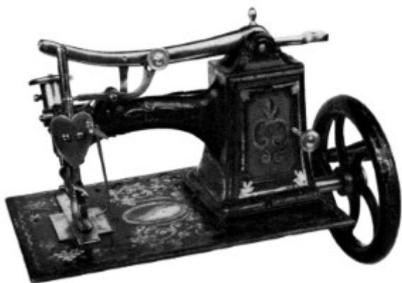
Figure 95.—[A.C.] HERRON'S PATENT SEWING MACHINE, 1858. The manufacturer of this machine is not known, but the
