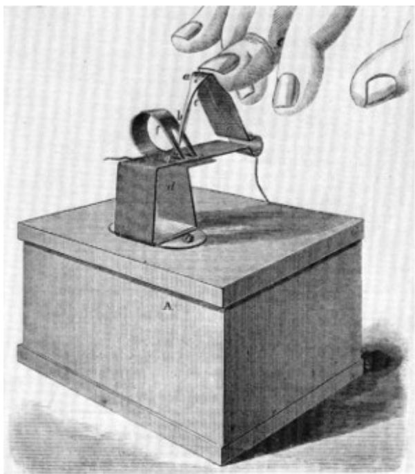
Figure 49.—HEYER'S MACHINE as illustrated in Scientific American , July 30, 1864. The smallest and most original of all the attempts to simplify machine sewing, Heyer's machine, which made a
