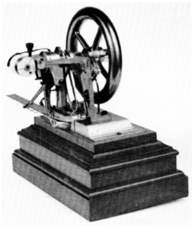
Figure 15.—HOWE'S PATENT MODEL, 1846. (Smithsonian photo 45525-B.)
