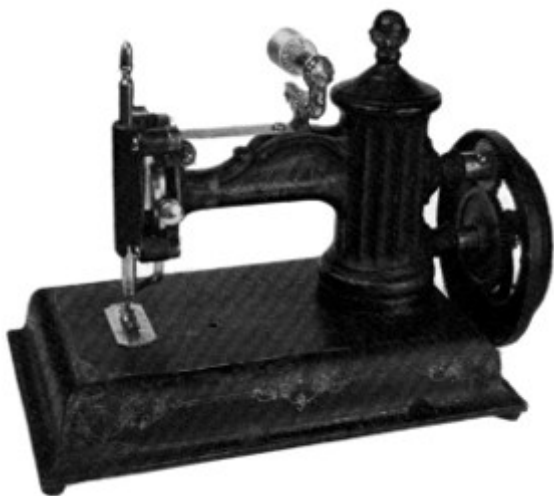
Figure 84.—GLOBE SEWING MACHINE. J. G. Folsom received two design patents in 1864, one on March 1 for a spool holder and one on May 17 for the basic style of the machine. Also in the same year, he was awarded a mechanical patent for an adjustment in the lower looper that would accommodate a change in needle size. Using
