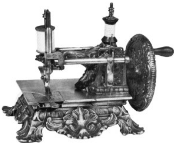
Figure 111.—NETTLETON & RAYMOND SEWING MACHINE. One of the most ornate of the early, small, hand-turned sewing machines was patented and manufactured by Willford H. Nettleton and Charles Raymond whose first patent was received on April 14, 1857. The patent model, believed to be a commercial machine, is
