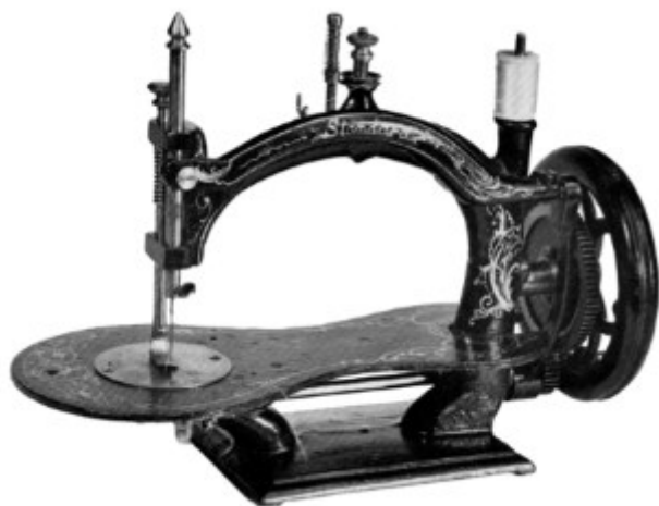
Figure 123.—STANDARD SEWING MACHINE of about 1870. This chainstitch machine is believed to have been made by the company that later became the Standard Shuttle Sewing Machine Company, when they
