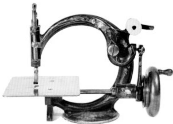
Figure 39.—ONE OF THE FIRST COMMERCIAL MACHINES produced by the Willcox & Gibbs Sewing Machine Co. in 1857, this machine bears no serial number, although the name “James E. A. Gibbs” is inscribed in two
