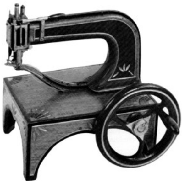
Figure 55.—BLAKE'S LEATHER-STITCHING MACHINE patent model of July 6, 1858; the inventor claimed the arrangement of the mechanism used and an auxiliary arm capable of entering the shoe, which enabled the outer sole to be
