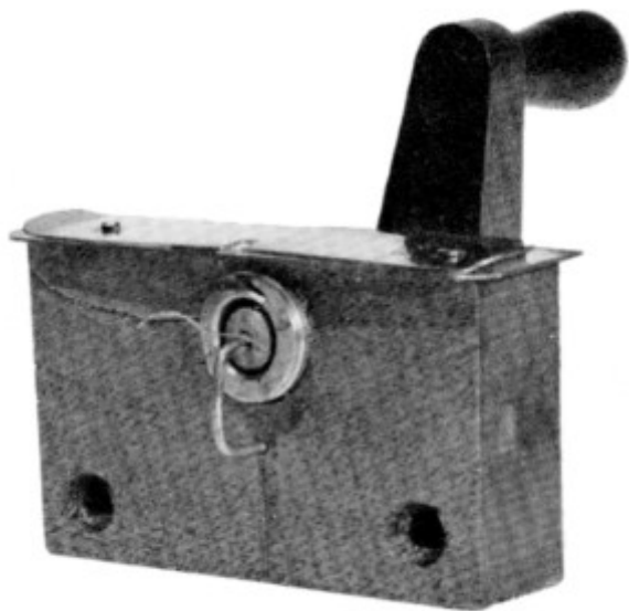
Figure 24.—WILSON'S PREPATENT MODEL for his rotary hook, 1851.
