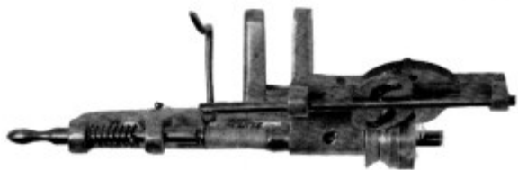
Figure 59.—SHANK'S patent bobbin winder, 1870.
