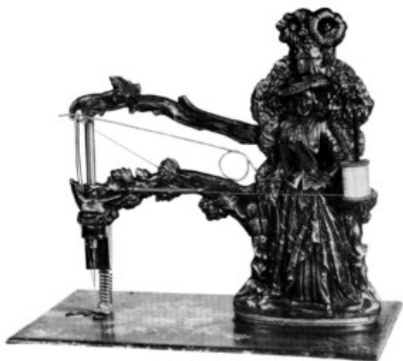
Figure 104.—“LADY” SEWING MACHINE of about 1859. The contemporary name of this machine is unknown. The unusual design of the head, or main support, is based in part on the design patent, number 216, of Isaac F. Baker, issued April 10, 1849, for a “new and useful design[,] for ornamenting furniture[,] called Cora Munro”
