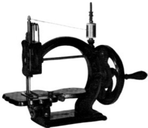
Figure 90.—GRANT BROTHERS SEWING MACHINE, 1867. This machine was one of several styles that utilized Raymond's 1861 patented chainstitch method.
