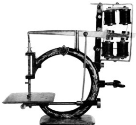
Figure 66.—JONES “ELECTRO MOTOR” PATENT MODEL of 1871 on a Bartlett sewing
