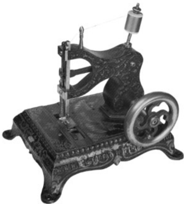
Figure 110.—NE PLUS ULTRA of about 1867. Another of the interesting hand-turned chainstitch machines of the late 1850s and 1860s was patented by O.L. Reynolds. The baster plates and the handle on the wheel are missing on this machine, but an
