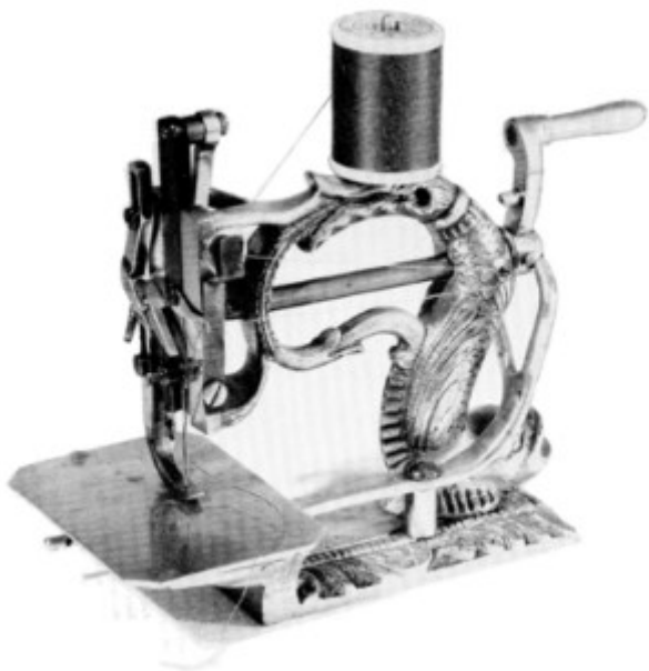
Figure 40.—A DOLPHIN sewing machine based on Clark's patent of 1858. This design was first used by T. J. W. Robertson in 1855, but in his patent issued on May 22 of that year no claim was made for the machine design, only for the
