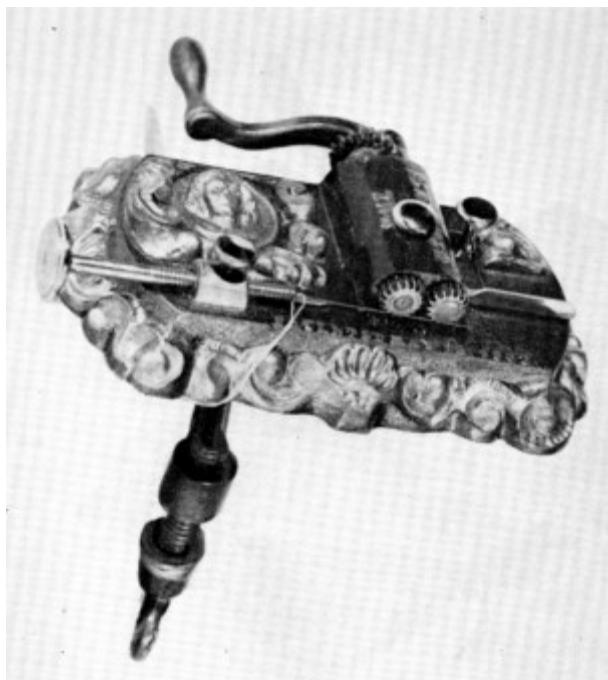
Figure 52.—THE FAIRY SEWING MACHINE sold for five dollars and was adequate for its advertised purpose, sewing or running very lightweight fabrics. The machine was marked with the Palmer patent, the date
